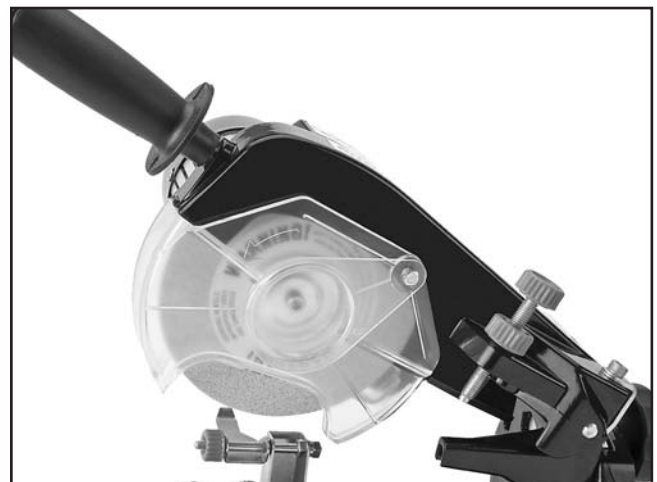
Figure 13. Grinding wheel and safety guards installed.
